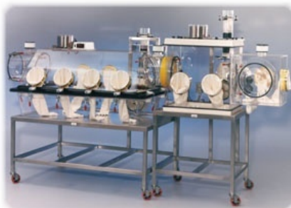
glove box to prevent emission of unwanted contaminants (www.plas-labs.com)
