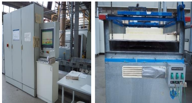
Figure 1: A laboratory-made hot air dryer (left) and over- and under- flow drying compartment (right).
